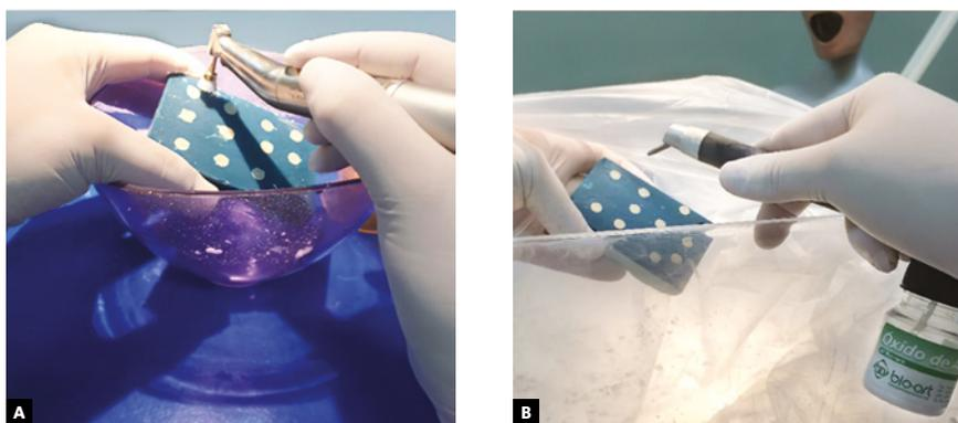
**Figure 2** - Photographs of the surface treatment process: **A)** surfaces polishing with pumice slurry; **B)** sandblasting of the samples with 50-µm Al<sub>2</sub>O<sub>3</sub> particles.
