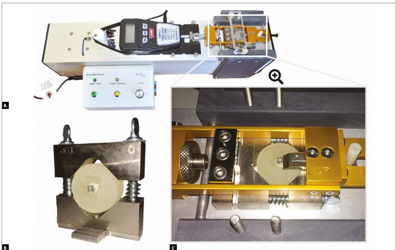
**Figure 3** - **A)** Image showing the Shear Bond Tester® device in a panoramic view. In **(C)**, it is possible to observe a photographic close-up of the area where the machine generates the shear force on the bracket, which is bonded to a cylindrical sample of provisional prosthetic material, until the adhesive failure occurs. In **(B)**, it is possible to observe the test object, which is held by the specially designed support of the machine.
